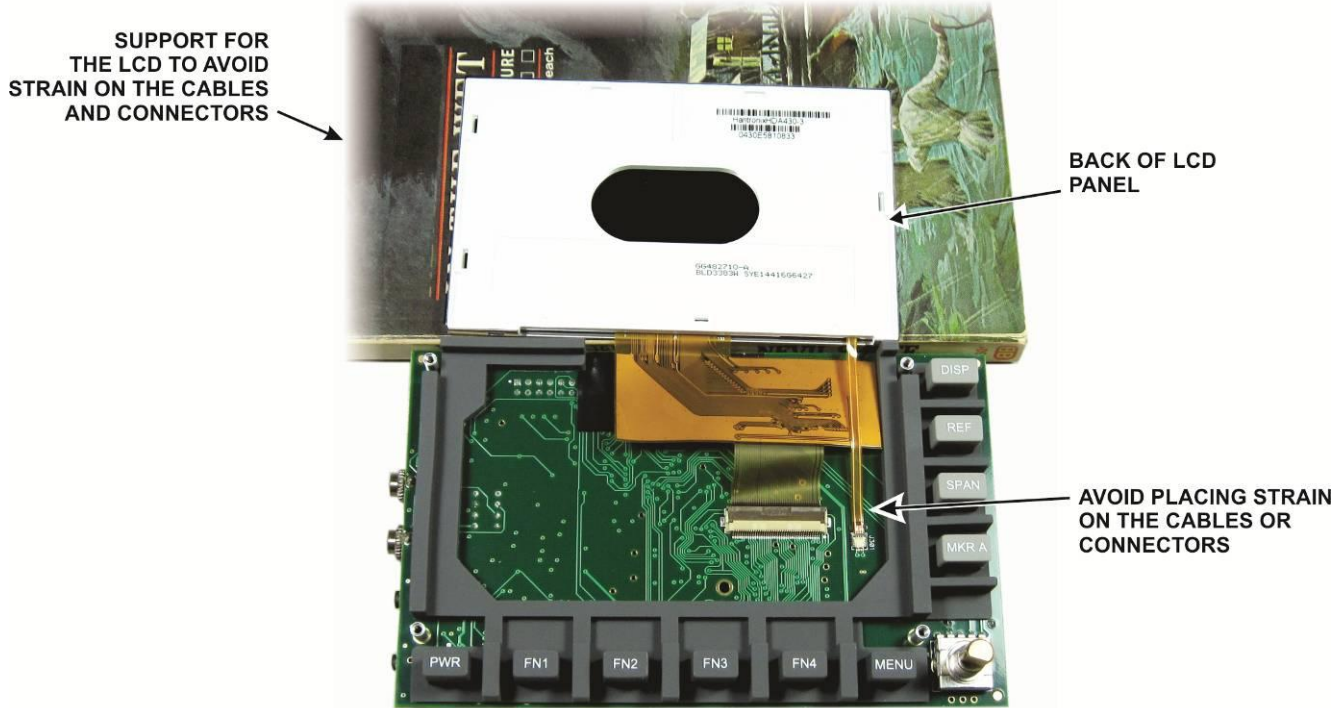
Figure 47. Removing LCD Panel from Rubber Key Matrix.
